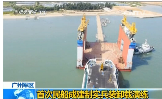
Semi-submersible barge used with offshore mobile debarkation system in 2014 exercise (CCTV)
